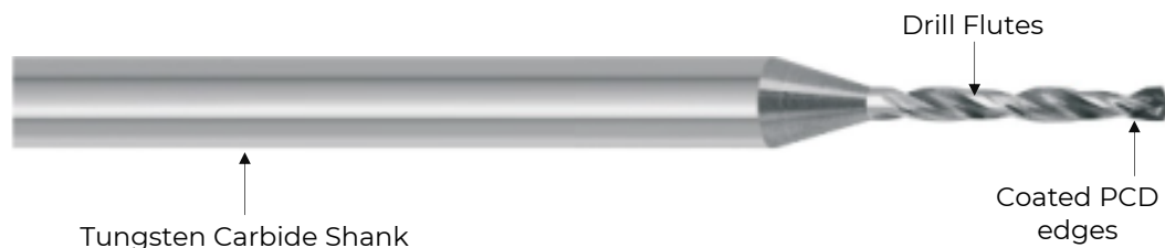
Figure 2-5. Example of the polycrystalline diamond micro-drill bit
